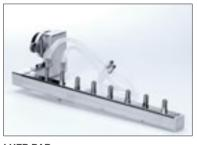
**LUER BAR** Equipped with 9 luer locks male, 2 plugs for voluntary injectors, 2 silicon hoses with 1 luer lock female and 1 luer lock male on each end. Fine filter is included. Art. no: 502951800
